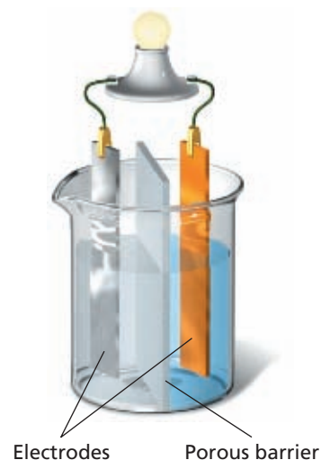
FIGURE 3 The light bulb is powered by the reaction in this cell.
