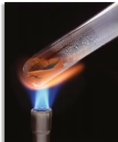
FIGURE 1 When heated, mercury(II) oxide decomposes into its elements, mercury and oxygen. Liquid mercury reacts with oxygen to re-form mercury(II) oxide. Together these reactions represent a reversible chemical process.
