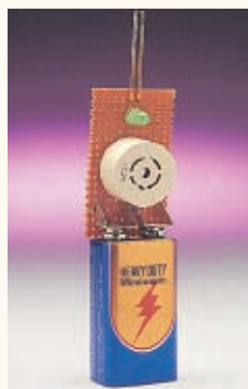
Teacher-made LED conductivity tester
