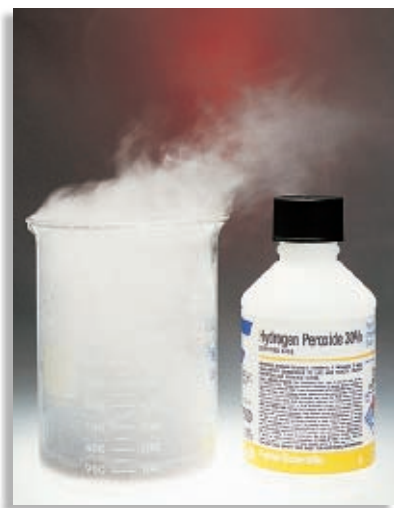
FIGURE 8 The reaction rate of the decomposition of hydrogen peroxide, \text{H}_2\text{O}_2 , can be increased by using a catalyst. The catalyst used here is manganese dioxide, \text{MnO}_2 , a black solid. A 30% \text{H}_2\text{O}_2 solution is added dropwise onto the \text{MnO}_2 in the beaker and rapidly decomposes to \text{O}_2 and \text{H}_2\text{O} . Both the oxygen and water appear as gases because the energy released by the reaction causes much of the water to vaporize.
