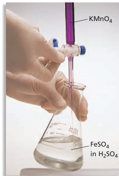
FIGURE 4 As a \text{KMnO}_4 solution is titrated into an acidic solution of \text{FeSO}_4 , deep purple \text{MnO}_4^- ions are reduced to colorless \text{Mn}^{2+} ions. When all \text{Fe}^{2+} ions are oxidized, \text{MnO}_4^- ions are no longer reduced to colorless \text{Mn}^{2+} ions. Thus, the first faint appearance of the \text{MnO}_4^- color indicates the end point of the titration.
