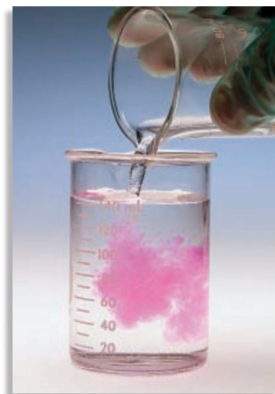
FIGURE 1 As NaOH solution is poured into HCl solution, a very rapid neutralization reaction occurs. Excess NaOH turns the phenolphthalein indicator pink.
