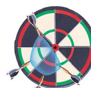
c Darts scattered around the target and far from the bull's-eye mean low accuracy and low precision.
