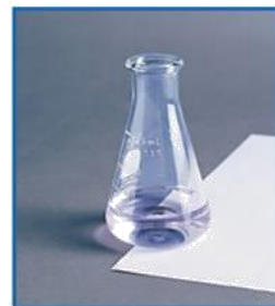
d When phenolphthalein is added to ammonia dissolved in water, a color change from colorless to pink occurs.
