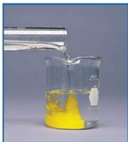
b When solutions of sodium sulfide and cadmium nitrate are mixed, cadmium sulfide, a solid precipitate, forms.
